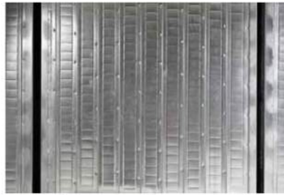
Figure 1. FIXCEL® metal core panel made of steel
